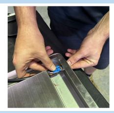
**Step 7:** Install the Push Button Switch into the 19mm hole, then flip the BBQ unit upright.
