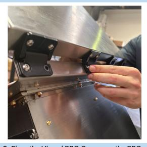
**Step 8**: Place the Hinged BBQ Cover over the BBQ plate and line up the holes on the black hinges with the holes in the fold of the S/S Support Plate. Insert the S/S Security Bolts and tighten the locking nuts using the tool supplied.
