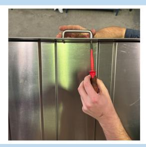
**Step 9:** Install the S/S Handle on the front of the lid by screwing the hardware supplied through the holes in the aluminium heat shield.
