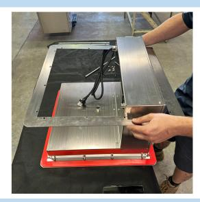
**Step 5:** Place the S/S support plate over the perimeter studs around the cooking plate. Make sure that the folded section of the support plate is facing to the rear of the BBQ with the fold facing downwards.
