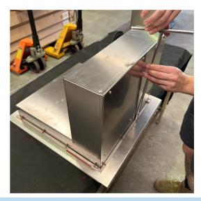
**Step 6:** Re install the 4 x S/S Escutcheon Support Bars, 16 x brass nuts and S/S tooth washers.
